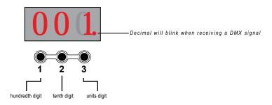
The decimal after the last digit will blink when the decoder is receiving a DMX 512 signal. If no signal is received the display will show the current DMX address and the decimal remains steady. If there is a wiring error or a short circut the display will show **ERR**.
